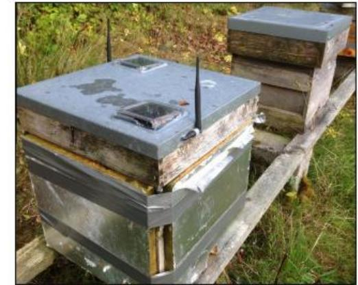
Fig. 3. Final instrumented hive at deployment site.
